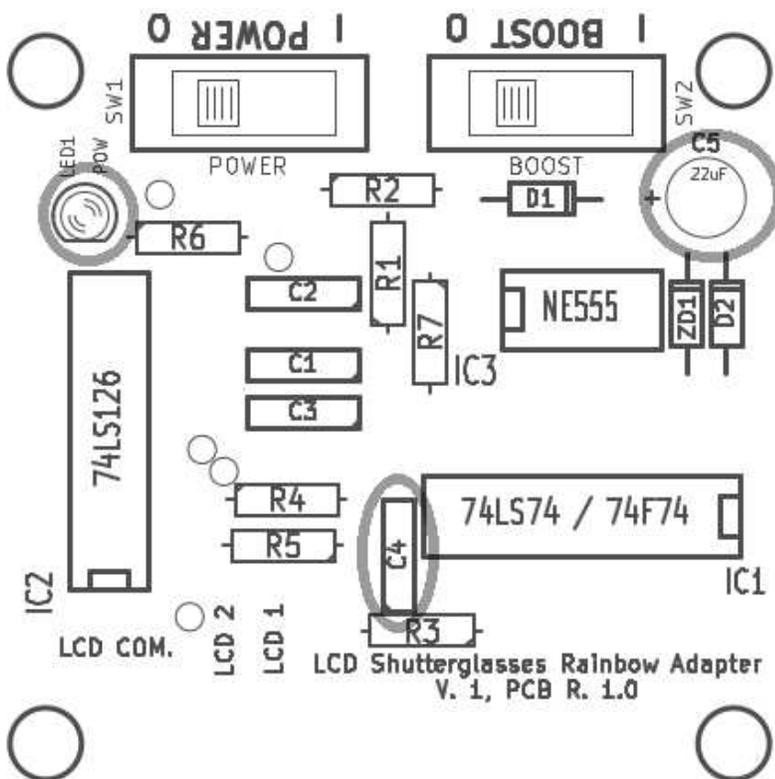
**Electrolytic Capacitors and LED: 4.7uF x1 (C4), 22uF x1 (C5), 3mm LED x1 (LED1)**
