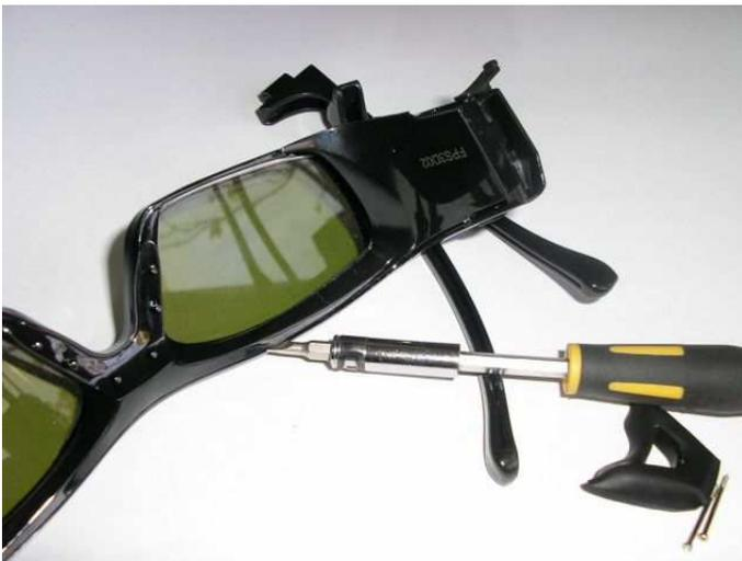
Once inside, the lenses on modern glasses seem often to be connected using a flexible PCB. On the SamSung glasses it was easy to solder the wires onto the solder pads connecting the lenses to the flex, then the
