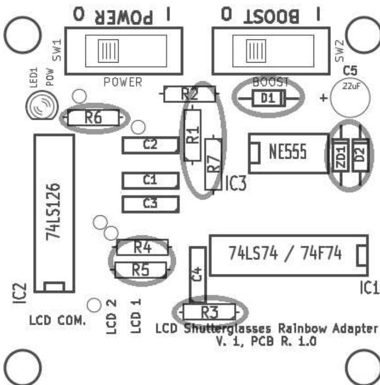
**Resistors and Diodes: R1 – R7, 1N4148 x2 (D1 – D2), 4V7 x1 (ZD1)**
