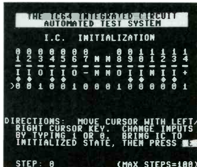
FIG. 6—THE FIRST TEST INITIALIZES each IC to a standard setup. The N shown for pin 11 indicates we don't care what the result will be on that particular pin.
